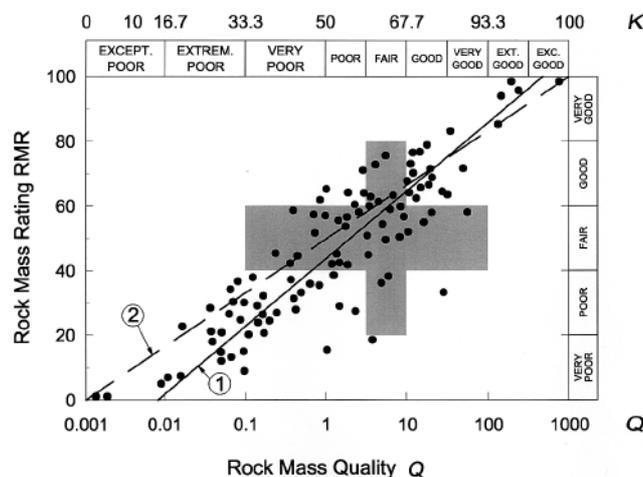
Figure 2: Different definition of the rock classes by two formulae.
