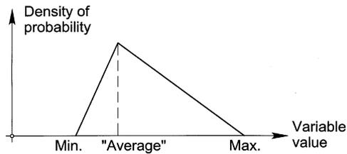
Figure 4: The usual triangular-shaped assumption for the density of probability for a Monte-Carlo simulation.
