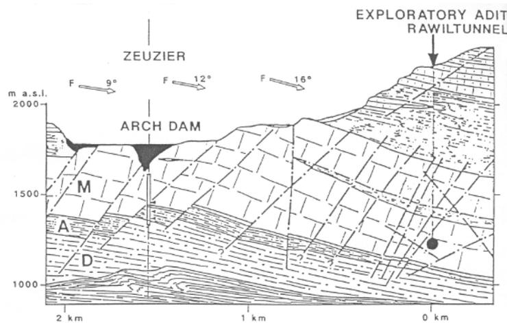
Figure 1: The excavation of the exploratory adit drained the ground water entrapped in layer D, caused the settlement of the region and damaged heavily the Zeuzier arch dam.
