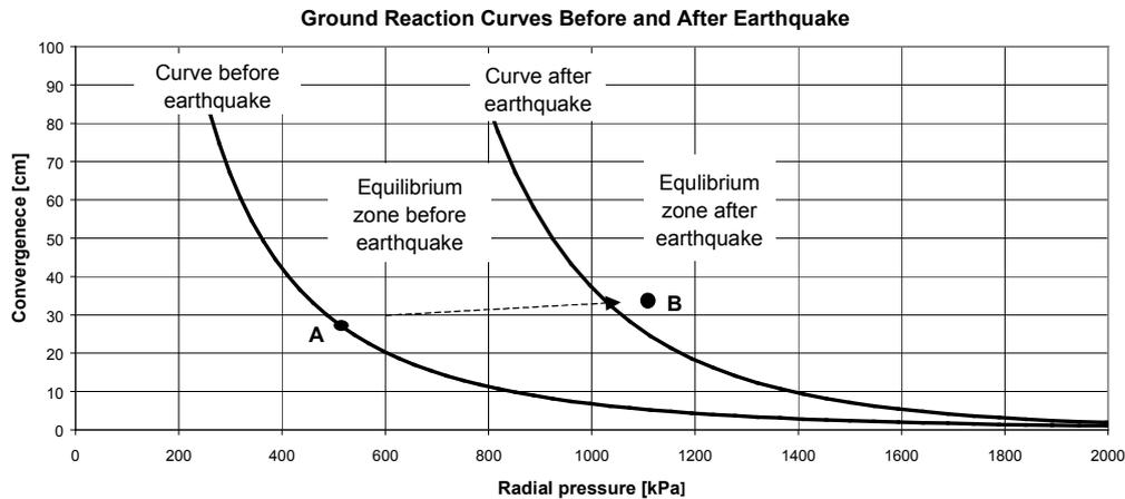
Figure 8 – Ground reaction curves before and after the design earthquake
