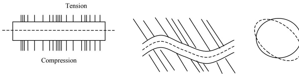
Figure a – Axial Compression      Figure b – Axial Bending      Figure c – X-Sect. Ovaling
