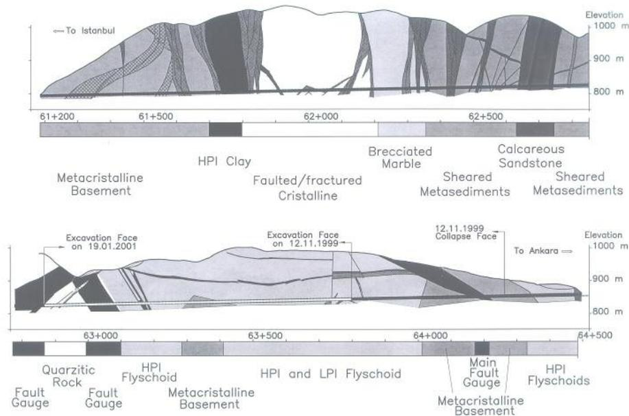
Figure 3 – Bolu Tunnel - longitudinal profile
