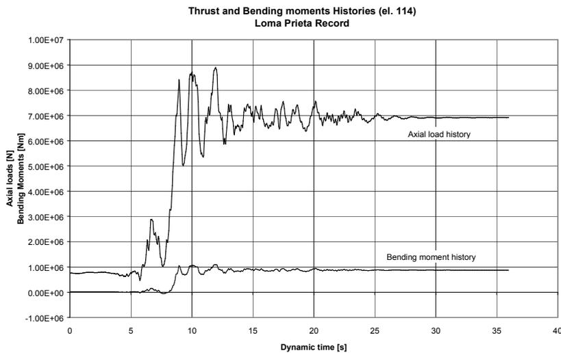
Figure 7– Typical thrust and bending moment history in inner lining
