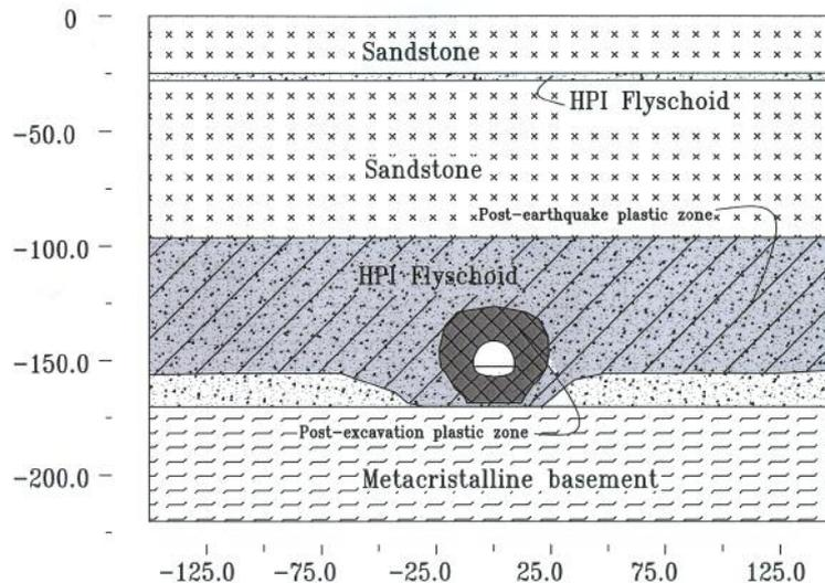
Figure 6 – Model grid, layering and extension of the plastic zones, after excavation and after the earthquake.
