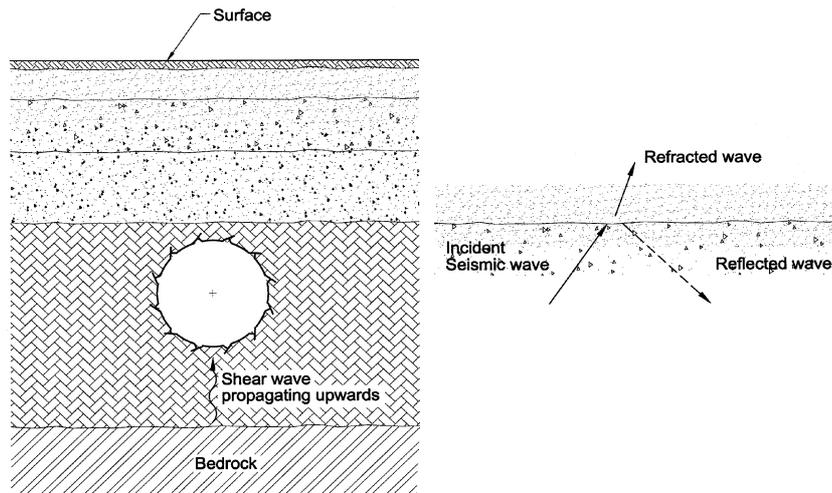
Figure 2 – Drifts induced by seismic shear.
