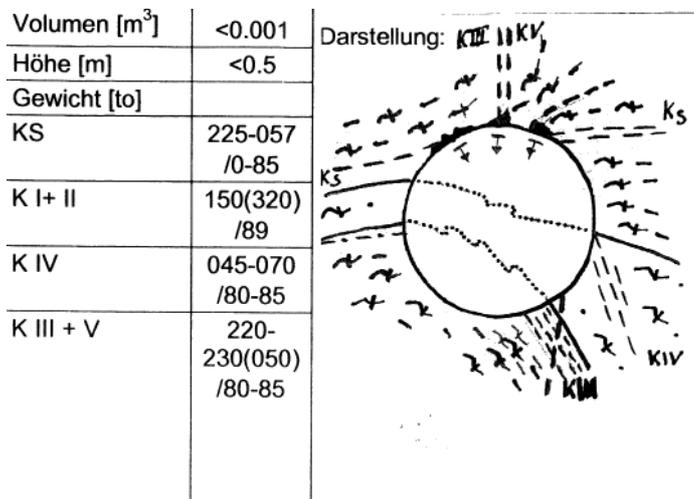
Figure 3. Tunnel mapping and potential modes of boundary failure reported for the western tube from ch. 13'569 to ch. 13'743.
