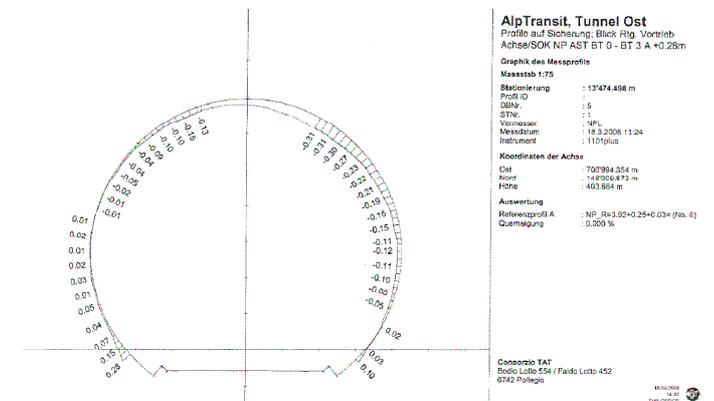
Figure 5. Convergences at chainage 13'474, eastern tube.
