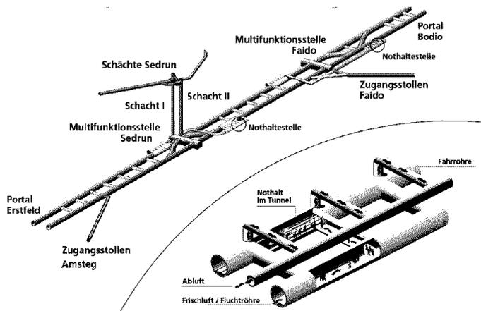
Figure 1. Gotthard Base Tunnel. Tunnel systems with shafts and adits.
