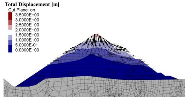
Figure 14. Permanent deformation of the dam for an MCE and empty reservoir (reservoir on the left side)
