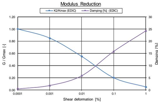
Figure 3. Shear modulus in function of the shear strain and the hysteretic damping.
