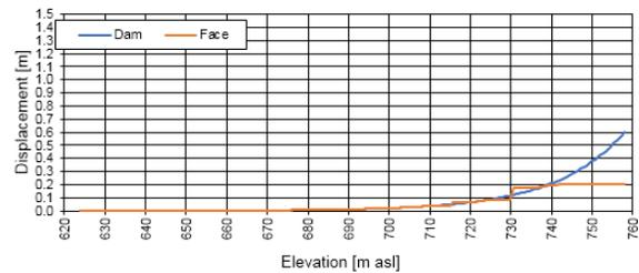
Figure 22. Displacement profile of concrete face and upstream face of dam in axial direction of the face
