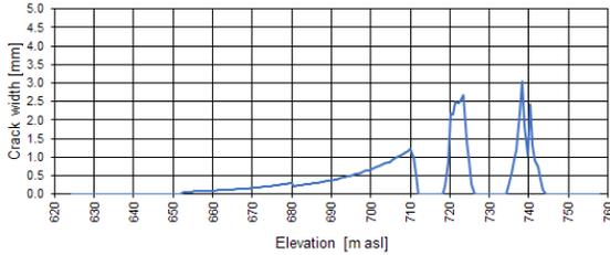
Figure 25. Profile of crack distribution and crack opening along the concrete face
