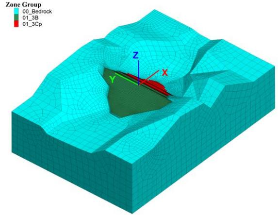
Figure 1. View on three-dimensional calculation model (downstream on the right, reservoir on the left)
