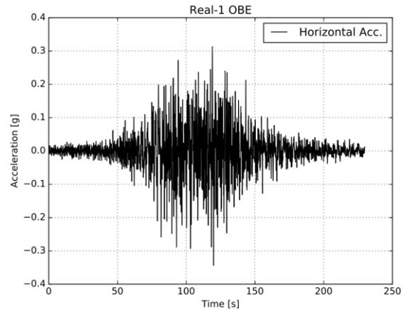
Figure 10. Horizontal input seismogram for the OBE
