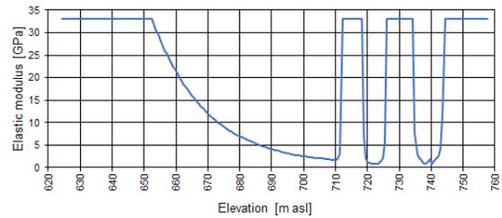
Figure 23. Profile of axial stiffness along the concrete face expressed as equivalent elastic modulus
