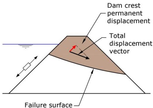
Figure 15. Permanent deformation of the upper part of the dam during strong motion in case of a full or nearly full reservoir.
