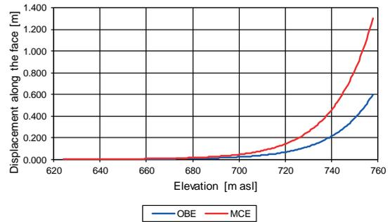
Figure 19. Displacement profiles along the concrete face
