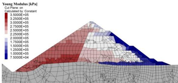
Figure 8. Elastic moduli of dam body materials after reservoir filling (reservoir on the left side)
