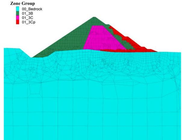
Figure 2. Cross-section of the three-dimensional calculation model (downstream on the right, reservoir on the left)
