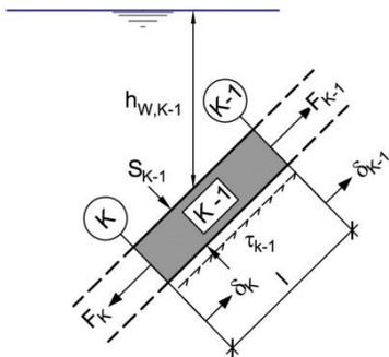
Figure 18. Equilibrium of forces and displacement at any point along the concrete face
