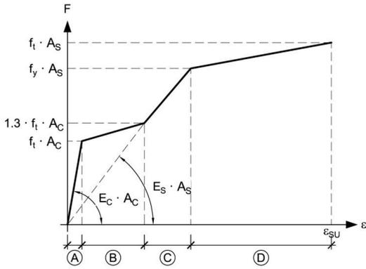
Figure 17. Axial stiffness of reinforced concrete
