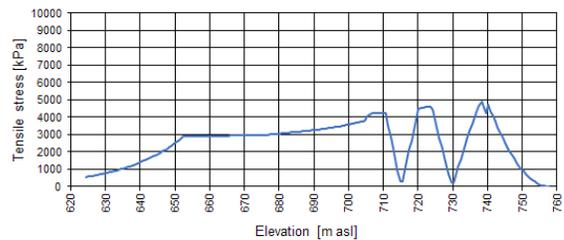
Figure 24. Profile of equivalent concrete tensile stresses along the concrete face
