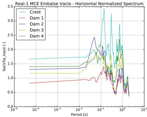
Figure 12. Spectral amplification of PGA for an MCE (horizontal component) – Empty reservoir
