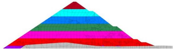
Figure 4. Construction phases of the dam as considered in the numerical model (reservoir on the left side)
