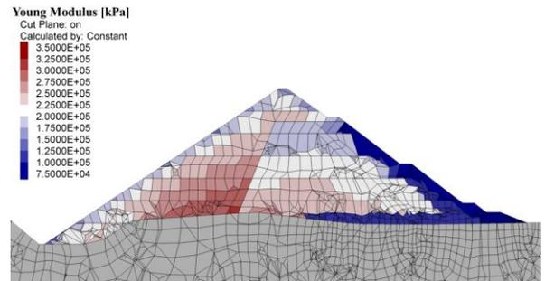
Figure 5. Elastic moduli of dam body materials at the end of construction (reservoir on the left side)
