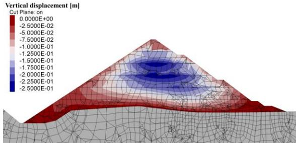
Figure 7. Vertical displacement at the end of construction (reservoir on the left side)
