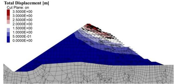
Figure 13. Permanent deformation of the dam for an MCE and full reservoir (reservoir on the left side)
