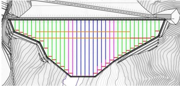
Figure 20. Concrete face with vertical and horizontal joints
