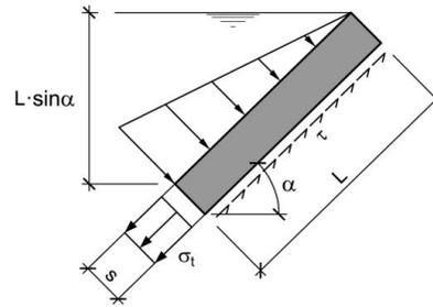
Figure 16. Scheme of the interaction between concrete face and dam body.
