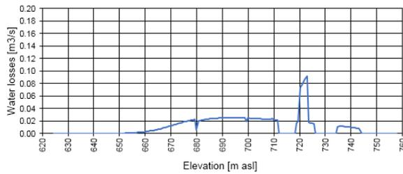
Figure 26. Profile of leakages along the concrete face
