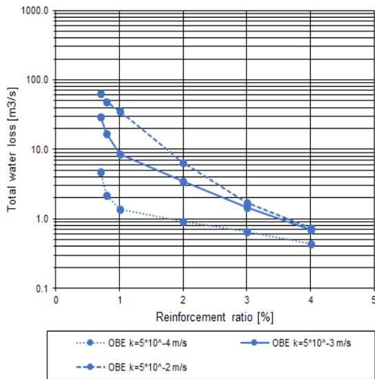
Figure 21. Leakages through concrete face as a function of reinforcement ratio and equivalent permeability of the dam material
