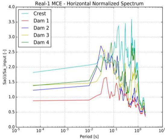
Figure 11. Spectral amplification of PGA for an MCE (horizontal component) – Full reservoir
