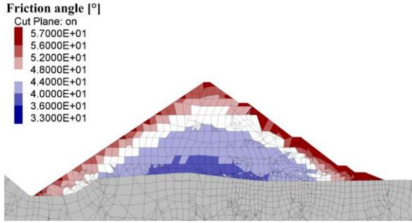
Figure 6. Friction angle of dam body materials at the end of construction (reservoir on the left side)
