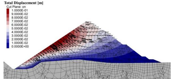
Figure 9. Total displacement of dam body after reservoir filling (reservoir on the left side)
