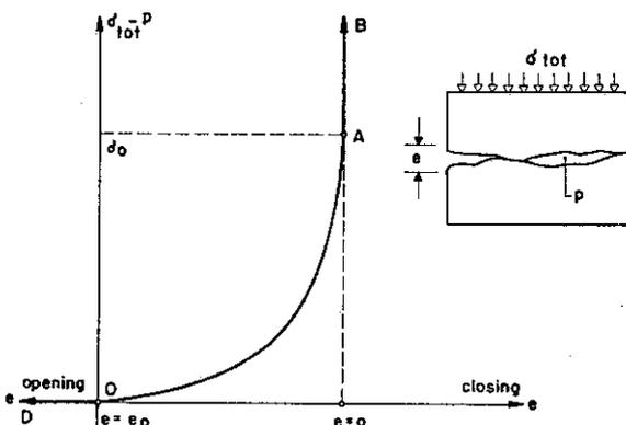
Figure 1 — Non-linear elastic opening of the joints due to internal water pressure according to F.E.S. - Model (Fissured, Elastic, Saturated Rock Mass-Model).
