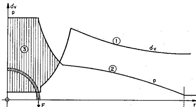
**Figure 5** — Equilibrium between water pressure and vertical stresses in the horizontal plane as an example.
