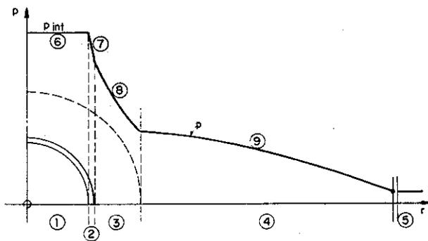
**Figure 4** — Example of distribution of water pressure around the tunnel.
