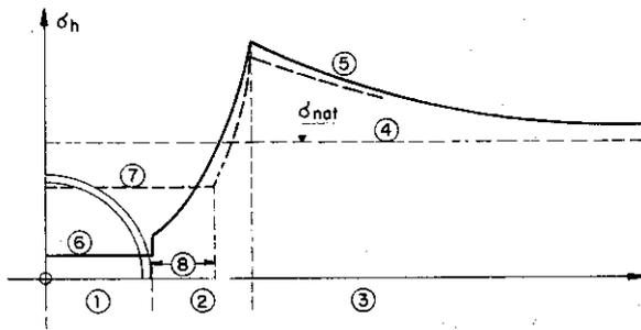
**Figure 3** — Empty tunnel in the drained rock mass; stresses in horizontal plane (assumed to be the critical one).
