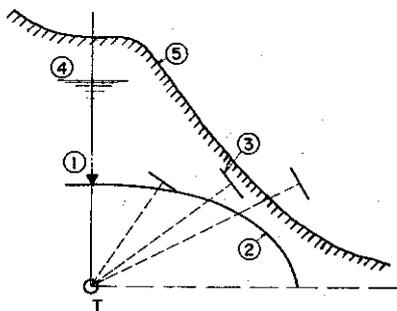
Figure 2 — Simple criteria to define the risk of hydrofracturing.
