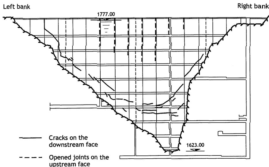
**Figure 3:** Damages of the Zeuzier arch dam caused by the settlement of the rock foundation.
