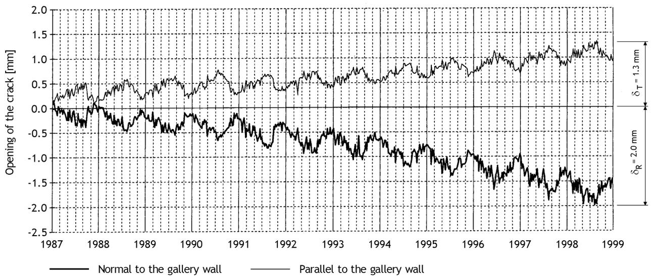
**Figure 12:** Opening of the downstream cracks measured at block 10.
