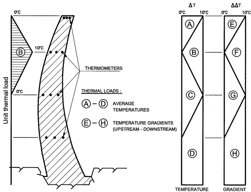
Figure 2: Unit loads for the thermal analysis.
