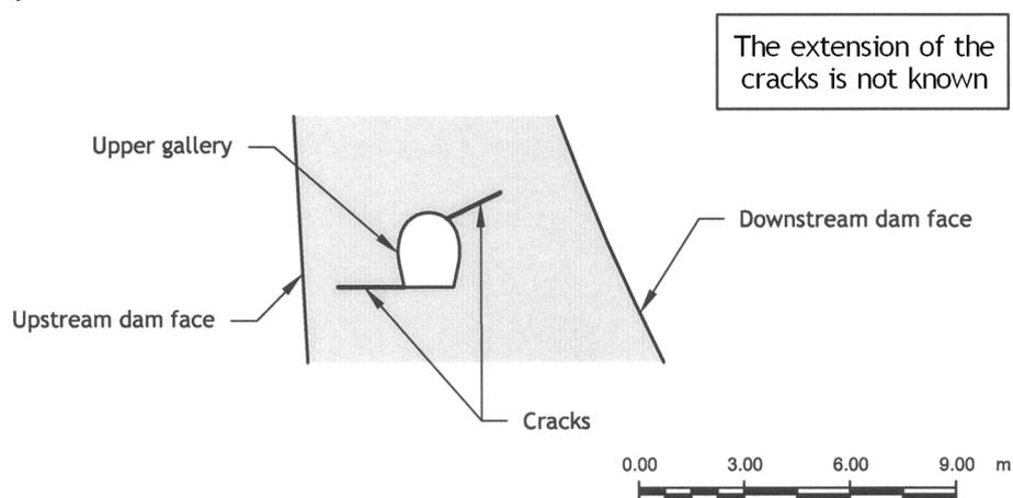
Figure 11: Schematic cross section showing the cracks of the Isola arch-gravity dam.
