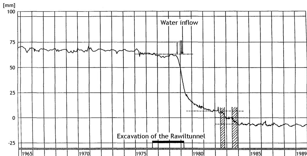
**Figure 7:** Reference radial displacements at the level of gallery 2.
