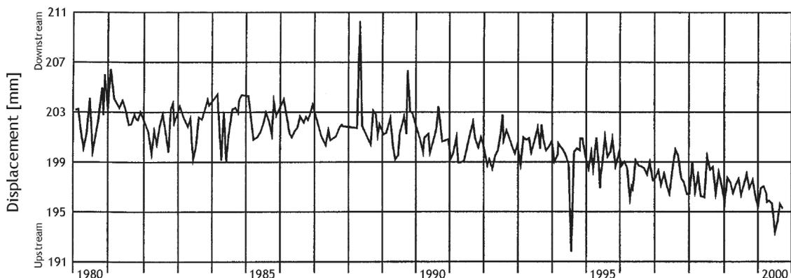
**Figure 14:** Reference radial displacement at the crest of the Roggiasca arch dam.
