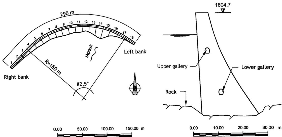
**Figure 9:** General layout of the Isola arch-gravity dam.
