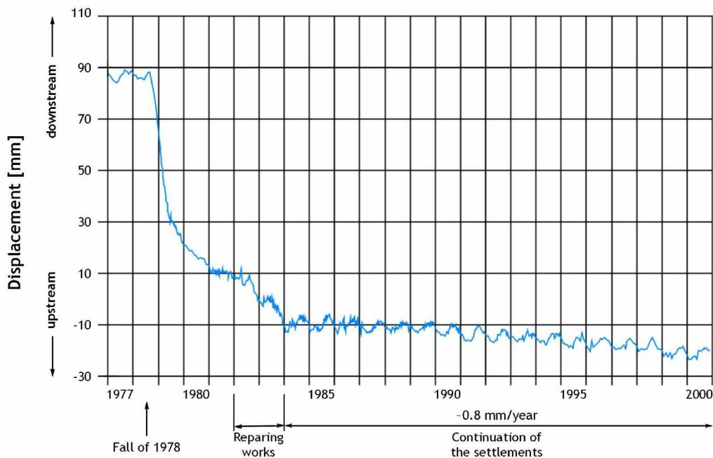
**Figure 8:** Evolution of the reference radial displacement at the dam crest since 1977.
