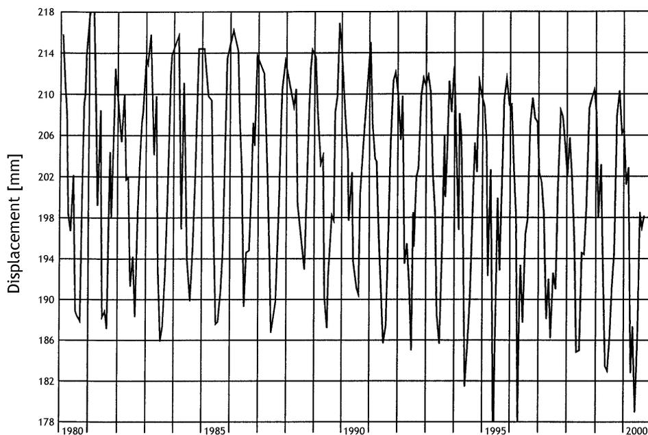
**Figure 13:** Measured displacements of the crest of the Roggiasca arch dam.
