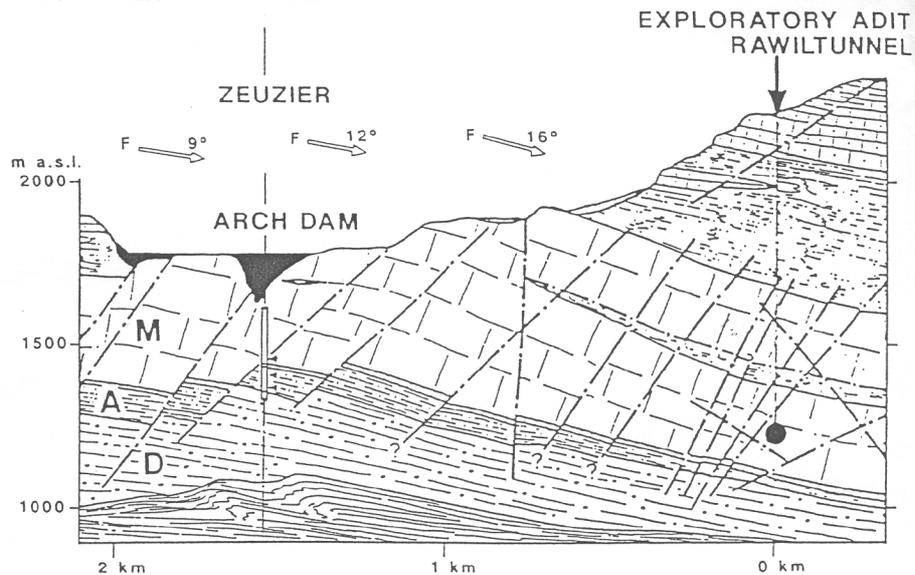
**Figure 4:** The excavation of the exploratory adit drained the ground water entrapped in layer D, caused the settlement of the region and damaged heavily the Zeuzier arch dam.
