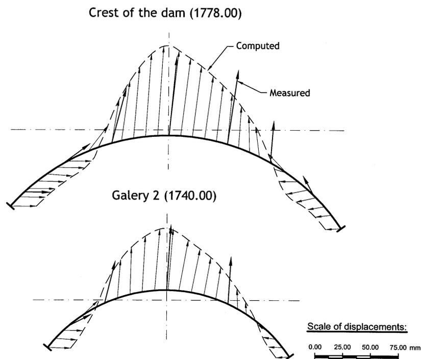
**Figure 5:** Measured and computed displacements of the Zeuzier dam.
