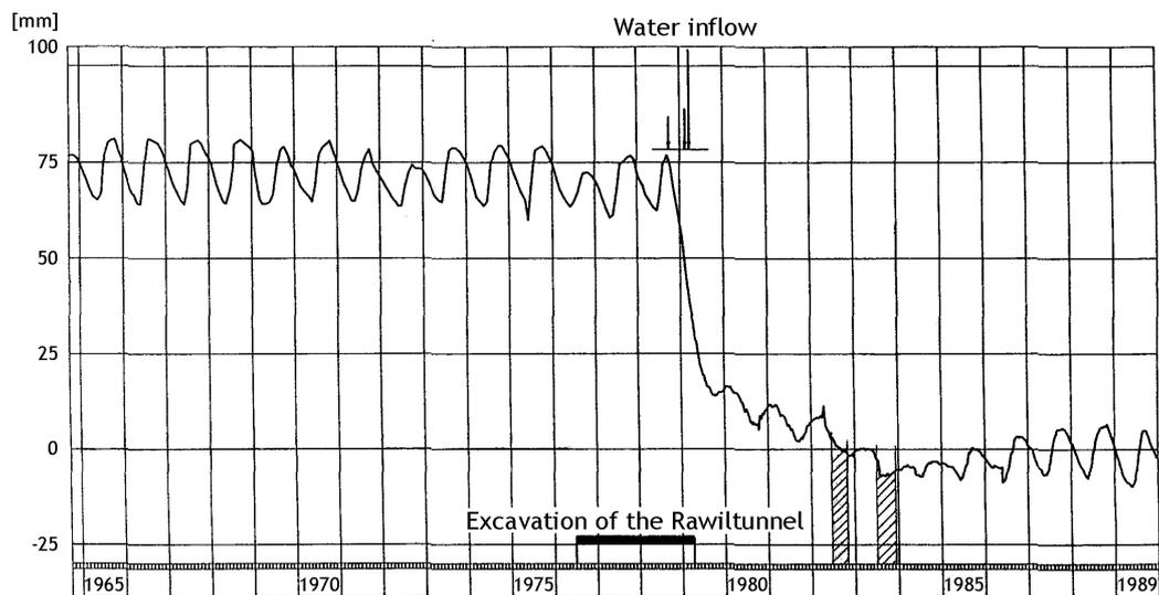
**Figure 6:** Radial displacements measured at the level of gallery 2.
