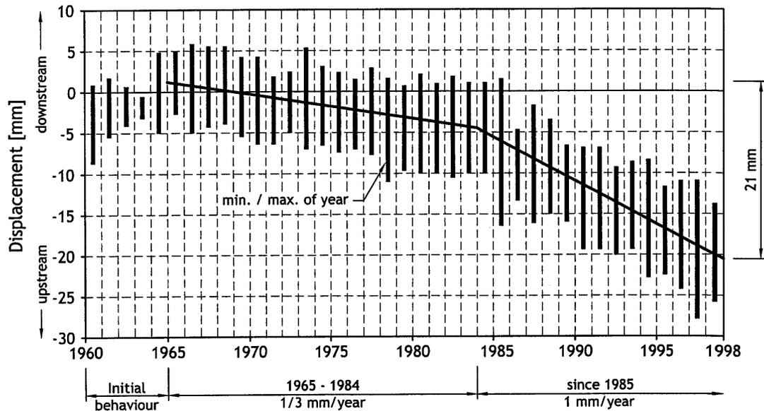
Figure 10: Evolution of the radial displacement of the dam crest since the construction (1960).
