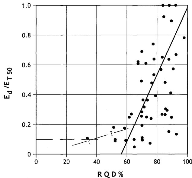
**Figure 1:** Relationship between RQD and a deformability factor defined as the ratio: modulus of deformability  $E_d$  to modulus of elasticity  $E_{T50}$  (Coon and Merritt 1970).
