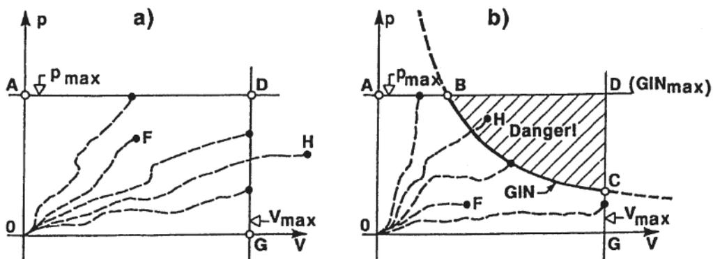
**Figure 16:** The limitations of the grouting process.
