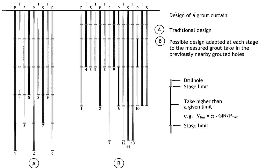
**Figure 24:** Design of a grout curtain.
