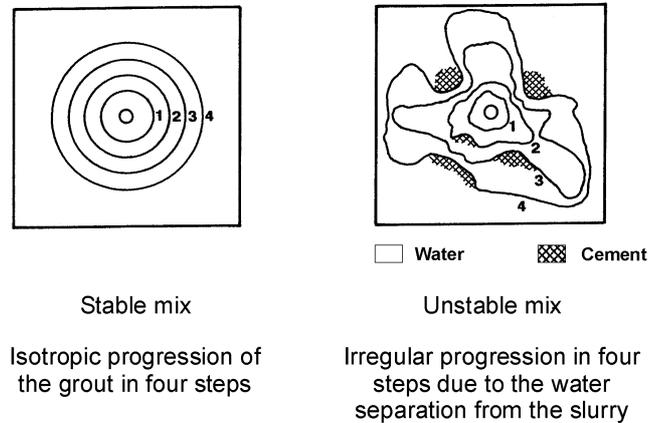
**Figure 7:** Experimental grouting tests in a joint of constant thickness (by Deere).
