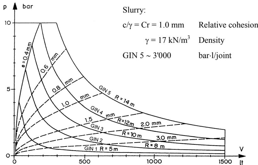
**Figure 17:** Example of grouting of a single joint.
