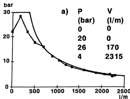
**Figure 18:** The GIN value is the governing factor of a hydro-jacking event. In this case an extremely high GIN value of 9000 bar·l/m was used.
