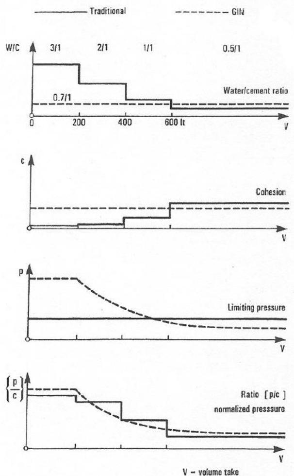
**Figure 22:** Comparison, by way of an example, of the traditional and the GIN grouting methods. The "normalised pressure"  $p_n = p/c$  is decreasing with increasing take, both for the traditional and the GIN method.
