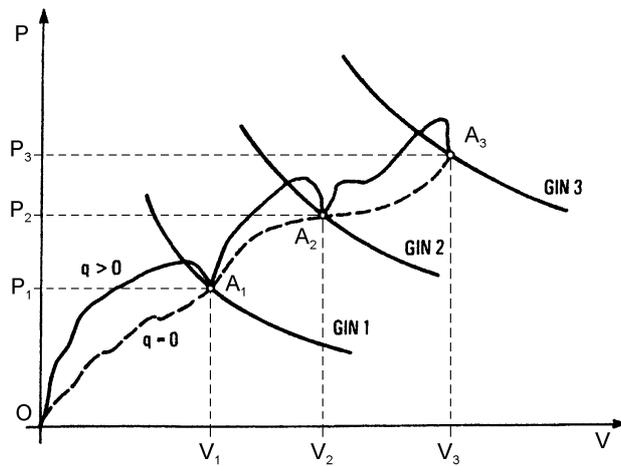
**Figure 15:** The grouting process can be stopped at any final pressure required or by reaching any required GIN value (there is no such situation as "refusal" by the rock). The successive values of GIN, represented by the rectangles  $O \cdot P_i \cdot A_i \cdot V_i \cdot O$  are an approximation of the energy  $E = \int_0^V p \cdot dV$  injected.
