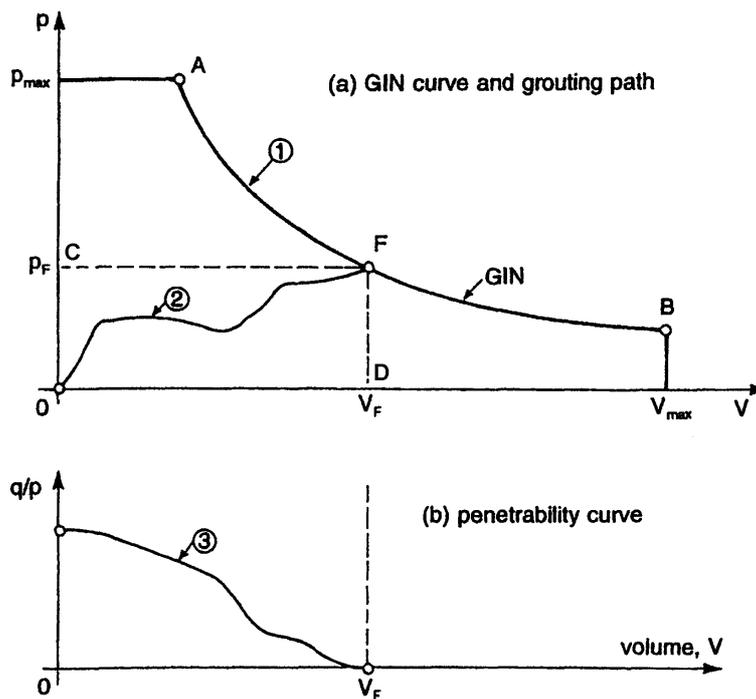
**Figure 21:** Grouting process of a single borehole stage (typical) where:
