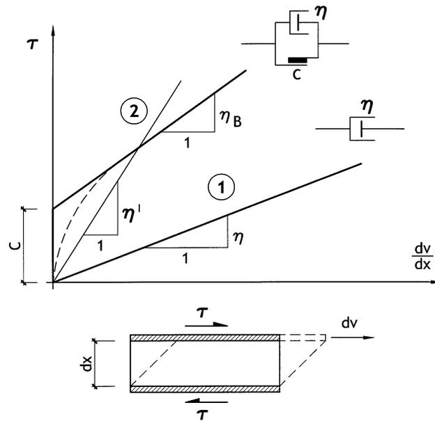
**Figure 8:** Rheology of a cement slurry vs water.
