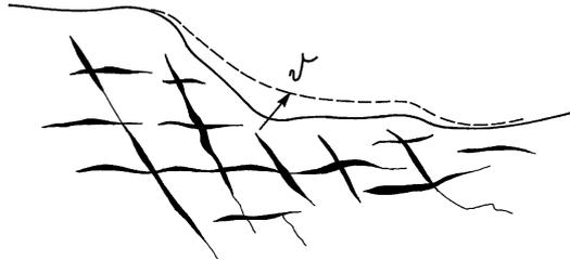
**Figure 10:** Unavoidable heave of the ground surface above a grouted zone.
